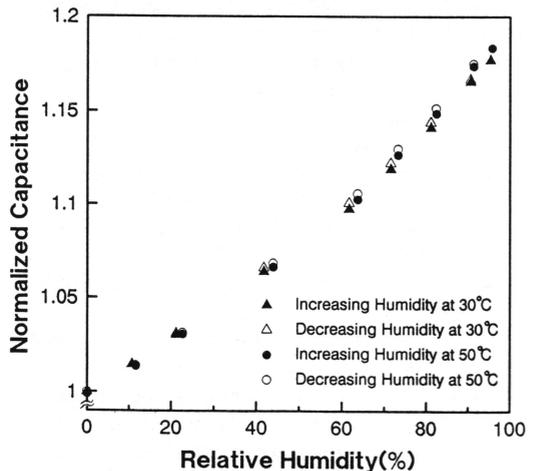
Fig.3 RH-C characteristics for CAB50
