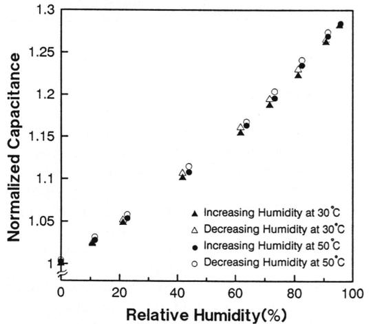
Fig.2 RH-C characteristics for CAB38
